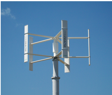
20 kW vertical wind turbine generator.
